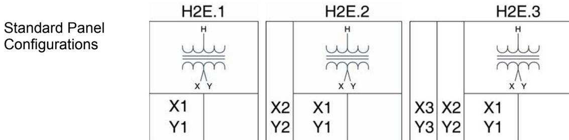
**Figure 1-13** Harmony-2E™ HMT Output Groups and Panel Configurations
