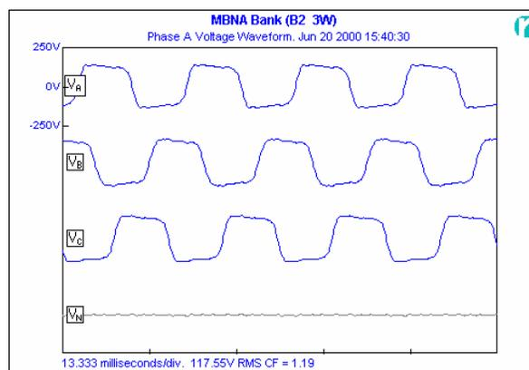
Figure 2: Voltage Flat-topping caused by 3<sup>rd</sup> Harmonic Blocking Filter
