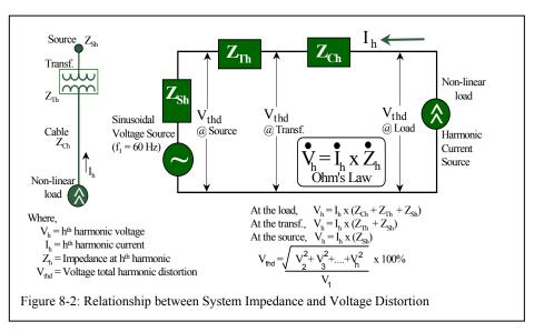
The fundamental is not a distortion component, so the RMS value of the distortion is just the square root of the sum of the squares of the harmonic components. Usually this is expressed as percentage of the value of the fundamental component and is called the *Total Harmonic Distortion*, or *THD*.
