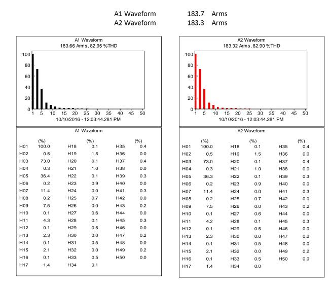
The actual current measured was close to the VFD/ASD max current rating at 60 Hz VFD operating speed. The current harmonic was quite high at approximately 83% of fundamental with a high triplen harmonic due to the single phase configuration of the source.
