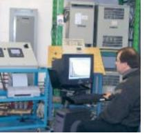
MIRUS products are factory tested under non-linear loading to ensure that the predicted performance and energy savings will be realized.
