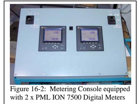
Figure 16-2: Metering Console equipped with 2 x PML ION 7500 Digital Meters
