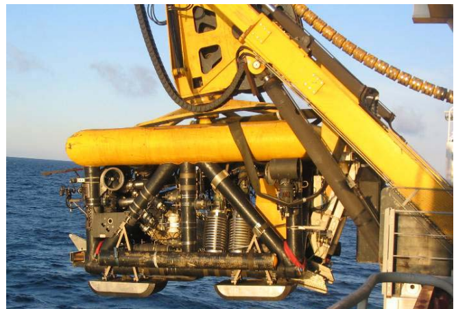
Fig. 17. Remotely operated pipeline trenching vehicle with 10 x 30kW thrusters and 4 x 300kW pumps
